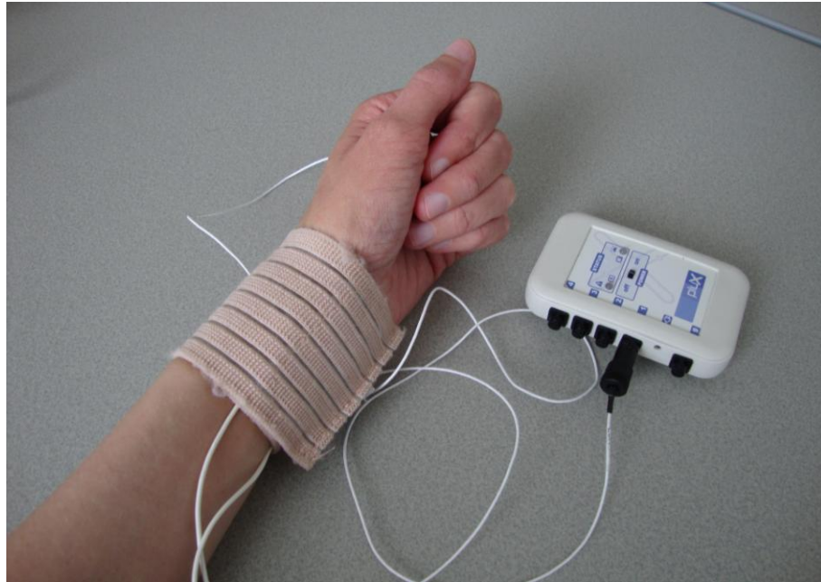
Figure 3.30: The bracelet, with the sensors underneath, on the left, connected to the PLUX device, on the right.
